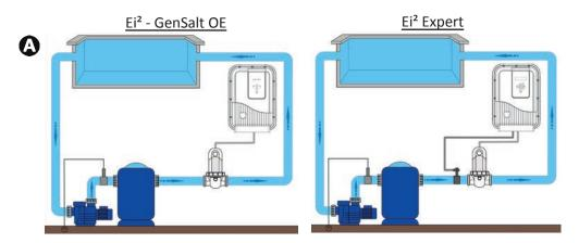
• The cell must be installed on a horizontal pipe to ensure an essentially horizontal flow of water through it, with no more than a 30 deg angle/slope. The pipe must have a free horizontal length of at least 30cm on which the cell will be installed. The cell must also be installed as far away as possible from any bends or elbows in the plumbing (B).
